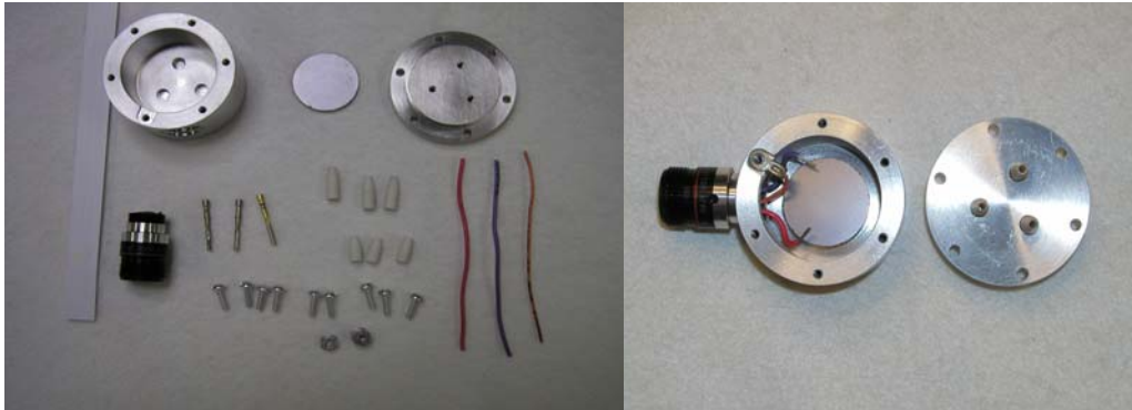
Figure 1. Silicon Calorimeter: (a) Components, (b) Partially Assembled Calorimeter
