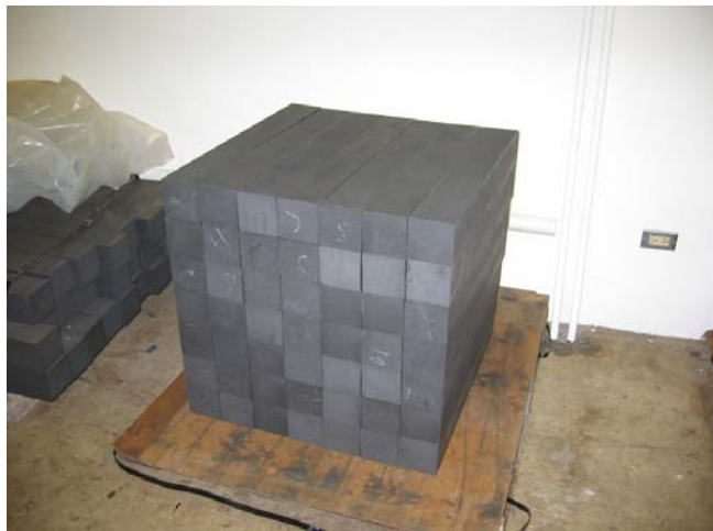
Fig 3. The 70 x 70 x 70 cm graphite cube that is used in the slowing-down-time experiment (left), and the shielded heating system that holds the graphite cube (right).
